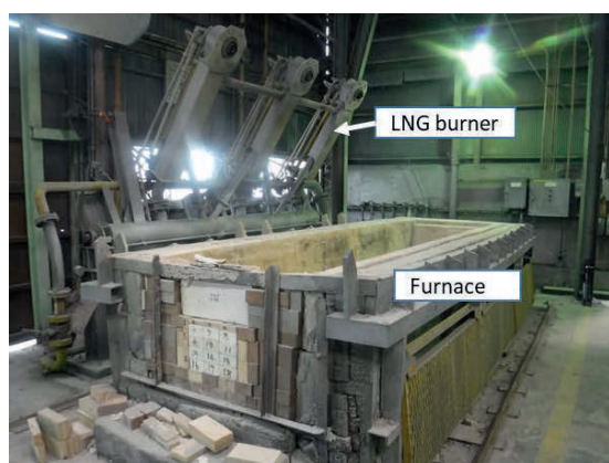
Fig. 8 Photo of experimental furnace for drying.
