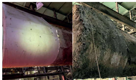
Fig. 4 Appearance of test material after demolding and test material after 5 months of use.
