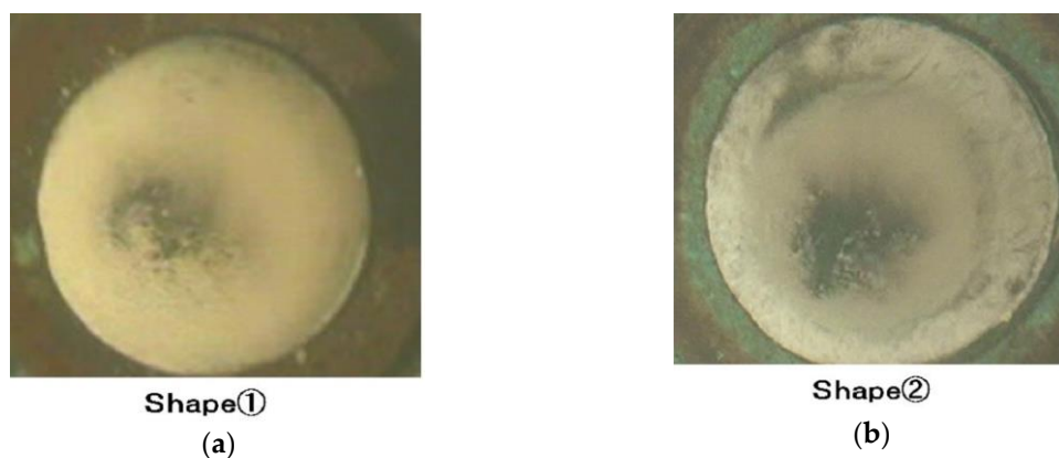
Figure 13. Comparison of the test results of water model simulation for the nozzle of Shape① (left) and Shape② (right) as the photograph taken from nozzle top with blowing gas.
