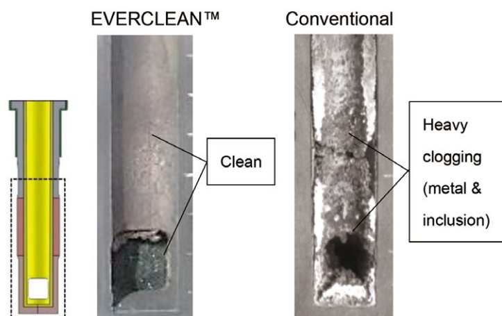
Fig. 2 Comparative photos after 3-heat casting of Al-Si killed steel
