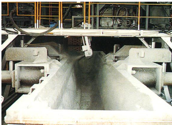
Fig.10 Automatic gunning machine for lining of TD (tundish) "TUNGUN".
