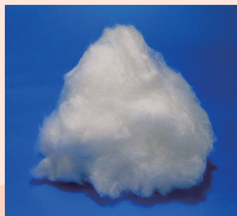
Photo 5-3 Biosoluble fiber "Super Wool" ®
