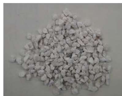
Photo 5-11 Used refractories after crushing and grading
