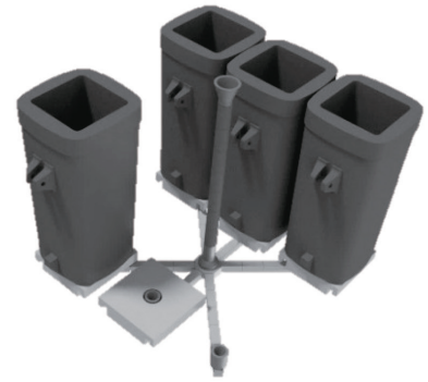
Fig. 9 Ingot casting -infographic-
