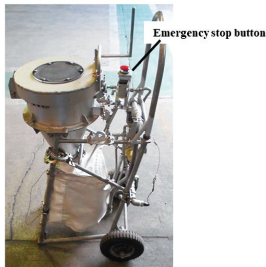
Fig. 4 Photograph of lightweight thermite welding apparatus
