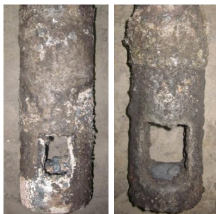
Fig. 3 Appearance of the SEN after casting (Left: used AG conventional product after 3ch., Right: used DG nozzle after 9ch.).
