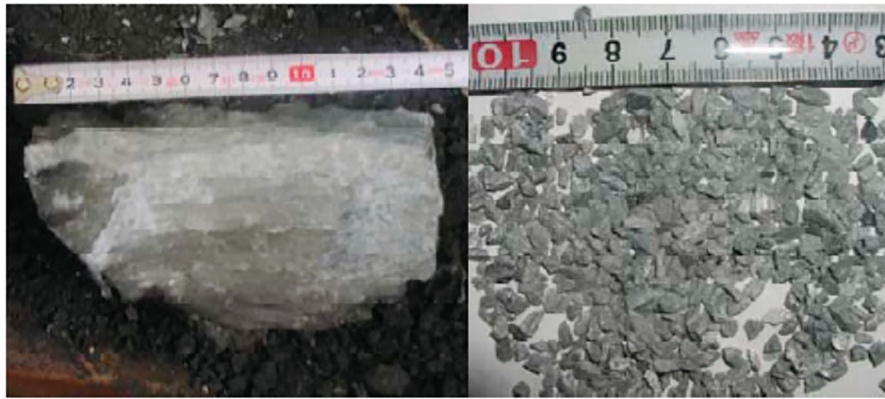
Fig. 1 Appearance of the synthesized material D. ( Left side : fracture surface of the ingot, Right side: grain of the material D )
