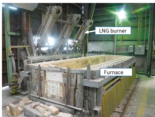
Fig. 8 Photo of experimental furnace for drying.
