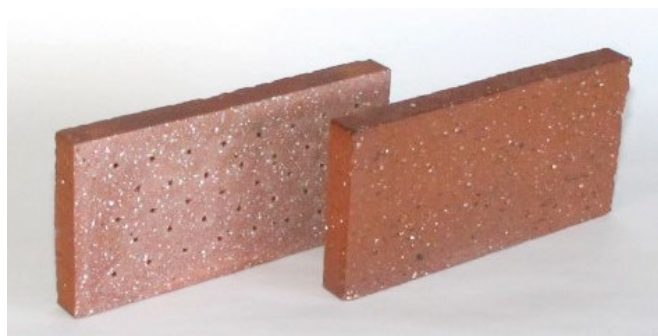
Fig. 2 Cross section of pervious bricks.
