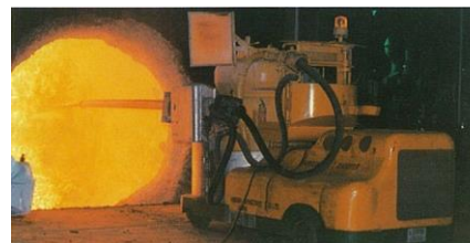
Unshaped refractories for converter blowing (The blowing is shown in the photograph above)
