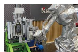
Robot replacing refractories for molten steel flow control
