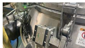
The opening of the mixer is equipped with a limiter switch, which prevents people from approaching while the mixer is in operation.
