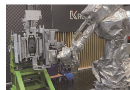
Robot replacing refractories for molten steel flow control
