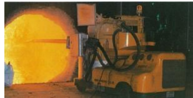
Gunning materials for converters (The blowing is shown in the photograph above)
